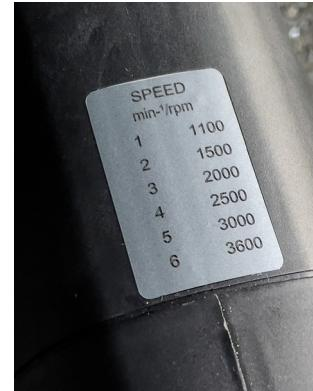
During operation, never increase the speed of the machine to above that of the maximum admissible speed of the grinding tool!
